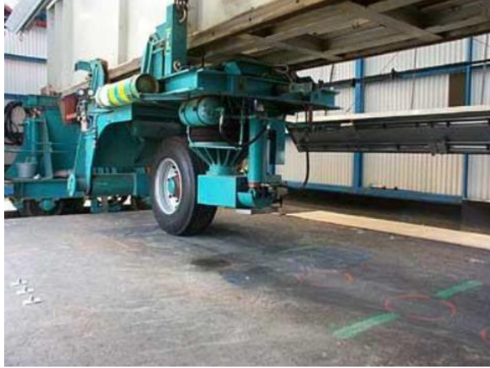
Figure 120: Delft University LINTRACK APT device.
