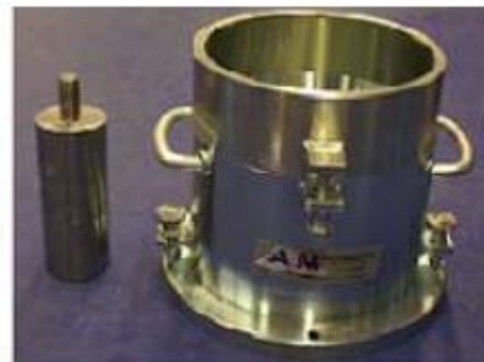
Figure 211: Repeated load CBR test setup for coarse grained granular materials (left) and test mold (right).
