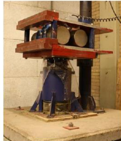
Figure 210: Delft University compaction device for preparing the \phi 300 mm, h = 600 mm triaxial specimens.
