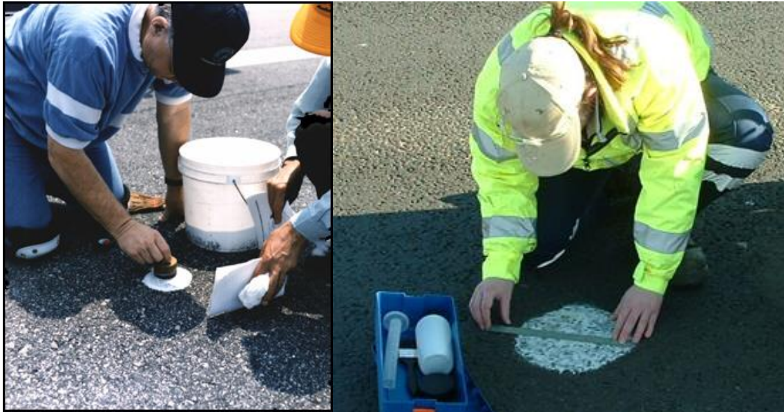
Figure 339: Sand patch test to determine texture depth.
