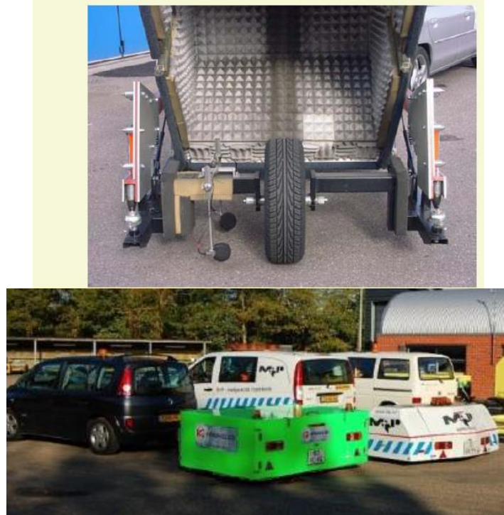
Figure 380: CPM method and CPM trailers. The top picture shows the inside of the trailer, note the microphones on the left hand side of the tire.
