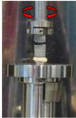
Figure 322: Stone – bitumen – stone column adhesion testing by means of the DSR.
