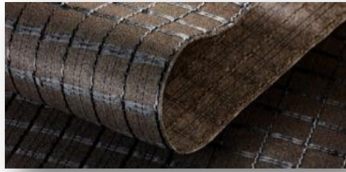
Figure 292: Composite system combining the function of a SAMI with that of a reinforcement.
