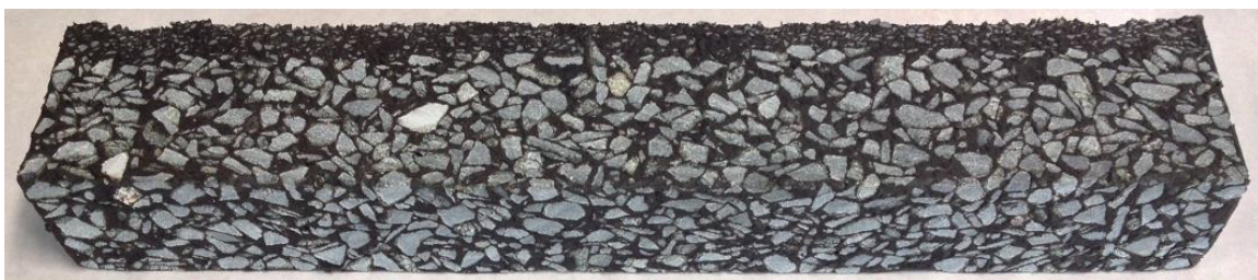
Figure 377: Bitumen-epoxy-silane-filler binder used in two layer noise reducing system.
