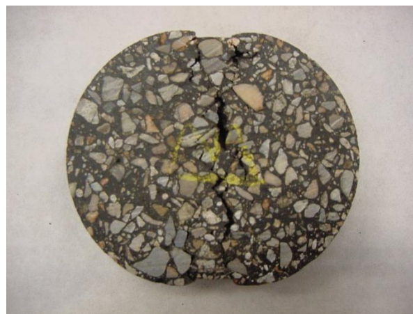
Figure 149: Indirect tension test specimen where loading strips have penetrated the specimen. Failure is a combination of shear, compression and tension.
