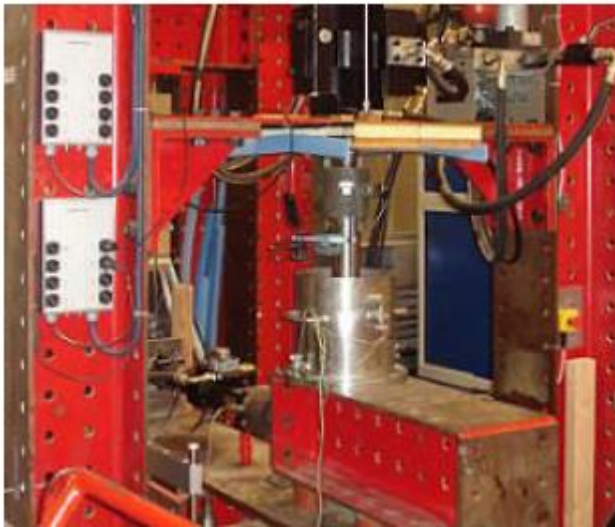
Figure 211: Repeated load CBR test setup for coarse grained granular materials (left) and test mold (right).
