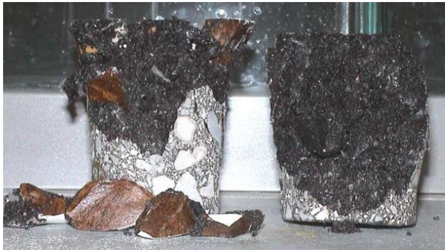
Figure 178: Adhesive cracking in a mixture made with crushed ceramic waste aggregate (left) and cohesive/adhesive cracking in a mixture with limestone aggregate.
