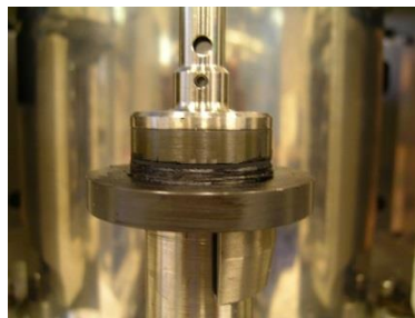
Figure 88: Principle of the dynamic shear rheometer test.
