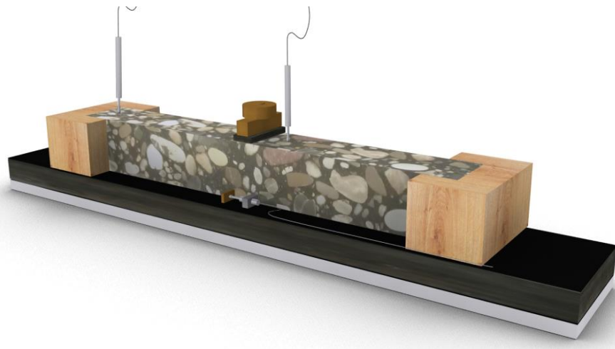
Figure 155: (a) The setup of the BOEF test and the haversine loading applied to the beam, where 0.05P is the preload. Where A: LVDT for vertical displacement; B: Beam 50 \times 50 \times 400 mm; C: Wooden C-Shape Support; D: LVDT for horizontal displacement; E: Latex sheet; F: Rubber foundation; G: Steel plate. (b) Artist impression of BOEF test setup.
