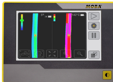
Figure 17: Number of roller passes and asphalt temperate shown as map.
