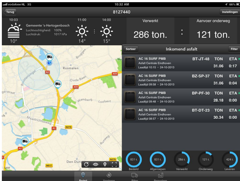
Figure 4: display with information about the asphalt trucks (Source: KWS (NL): ALIS: Asphalt Logistic Information System)
