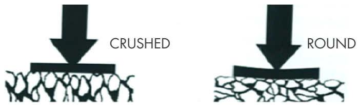
Figure 4b, Effect of aggregate shape
