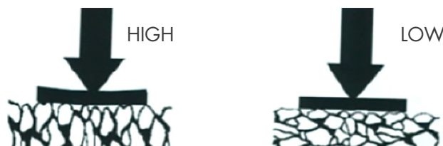
Figure 4a, Effect of aggregate flakiness
